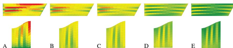
Figure 10: Balancing the fabrication requirements with the optimization. From left to right different optimization results are given by controlling the weights of constraints. First row is the top view and the second row is the side view of the last shell. Meshes are colored according to a maximal angle  $\kappa$  between the edges of neighboring faces. The comparison of  $\kappa$  angle,  $\alpha$  angle, and deviation from the target surface is given in Table 1.
