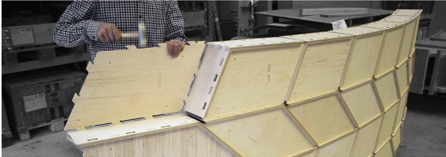
Figure 14: 4x7 segment prototype at scale 1:2.6
